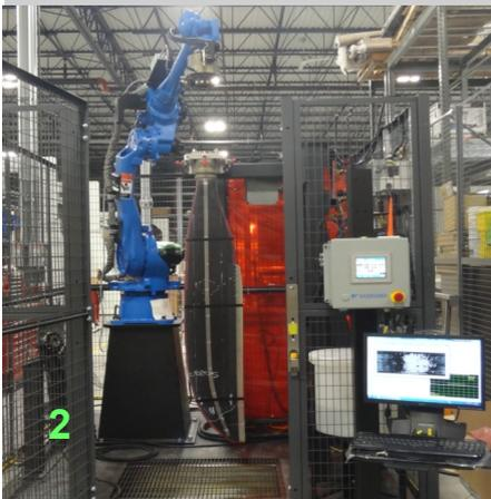
Following our first robotic installation earlier in the year at a GE Aerospace site (Fig 2), a further USL ultrasonic system has now been added to a robot for a different application (Fig 3). This will be used for thickness measurements on critical fabricated components as part of a precision manufacturing cell.
