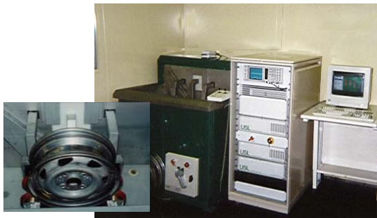
Automated system for measurement of weld penetration and undercut on car wheels (Ford Inc, Detroit)
